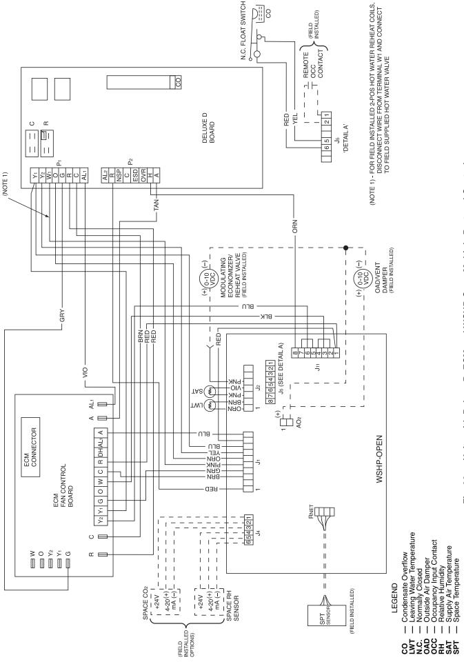
Fig. 28 — Units with Deluxe D, ECM and WSHP Open Multiple Protocol Controls
